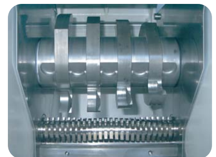
During routine cleaning, the rough crusher and granulator blades can be seen completely.
